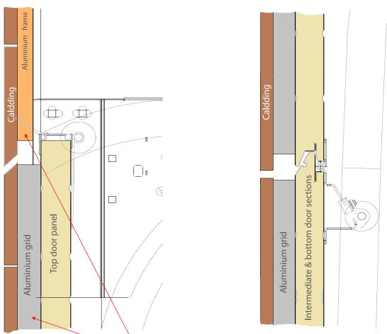
Aluminium frame installed in between the opening Aluminium grid for cladding fixing to the door
