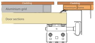
Aluminium frame with 180 mm lintel required. LHR-RM track system only.
